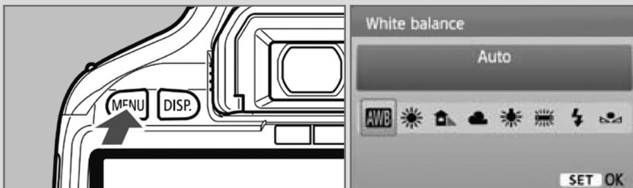
Press WB button, select the customer white balance on the display and confirm with the "set" button.
