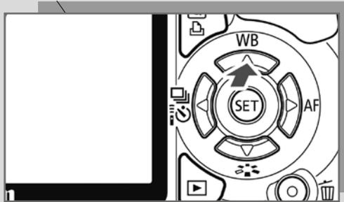
Please select the custom WB with the set-button and confirm the chosen picture with the set-button. We recommend naming the white balance picture taken with the DELTA®20 Plus/DELTA®20 accordingly.
