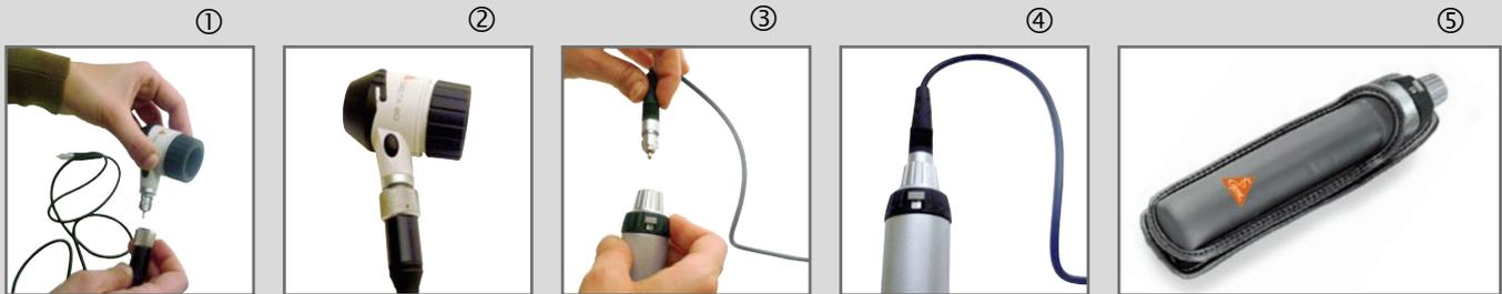
**4.** Connect the HEINE SLR Photo adaptor to the bayonet lock of the camera by placing the red or white spots on top of each other and twist to lock.
