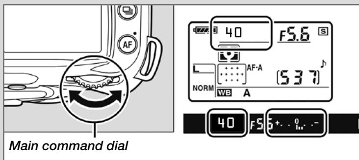
4. The white balance needs to be set once. To do this press the WB-button and turn the rear main command dial until "PRE" is displayed on the upper control panel.
