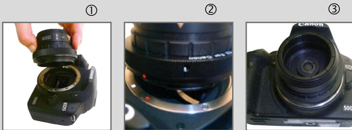
**5.** Connect the distance ring onto the line marked "Camera" on the focusing ring of the DELTA®20 Plus/DELTA®20 Dermatoscope head. Once attached, tighten the focus ring down until it makes contact with the distance ring.
